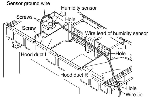
This illustration is under the condition which hood intake duct R is removed
